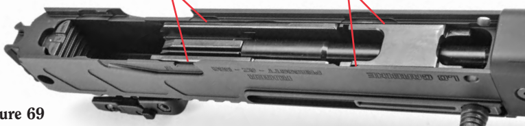
Apply Lubricant to Both Sides of Front and Rear Bolts
